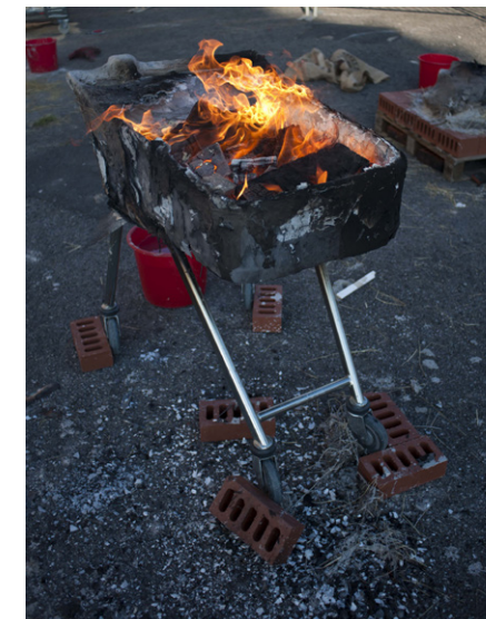
Left: Paper kiln in which clay items are surrounded with wood encased in layers of clay-soaked paper Middle: Kiln in a shopping trolley using paper kiln technique Right: Brick-built up draft kiln in which clay items are fired in a chamber above the fire
