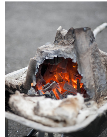
Left: Paper kiln in which clay items are surrounded with wood encased in layers of clay-soaked paper Middle: Kiln in a shopping trolley using paper kiln technique Right: Brick-built up draft kiln in which clay items are fired in a chamber above the fire
