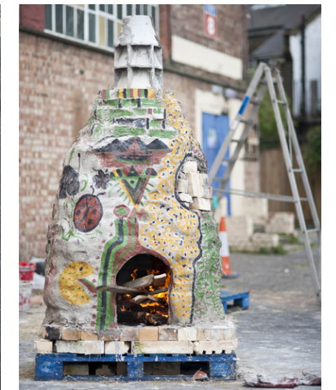
Left: Paper kiln in which clay items are surrounded with wood encased in layers of clay-soaked paper Middle: Kiln in a shopping trolley using paper kiln technique Right: Brick-built up draft kiln in which clay items are fired in a chamber above the fire
