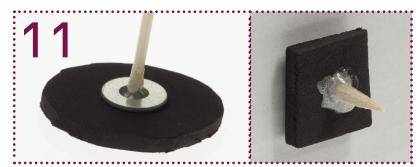
Tip: If the cam follower is not heavy enough to rest properly on the cam, attach a metal washer or nut like in the above picture to add a little weight.
