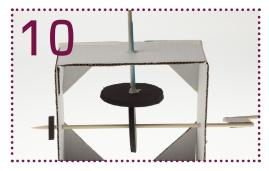
Move your cam so that it is under the cam follower. Then turn the handle of your automaton and adjust your cam until you get the motion you like (see step 4 for different placements). Once you have the right position glue the cam into place on the skewer stick axle.
